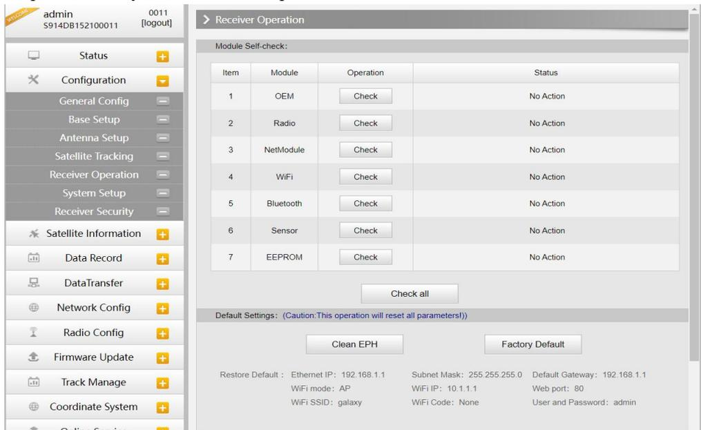
**Self-check:** Users can also do the self-check from this configuration page, click on the Check all button to check all the modems or click on the check button corresponding to the modem to check one by one.
