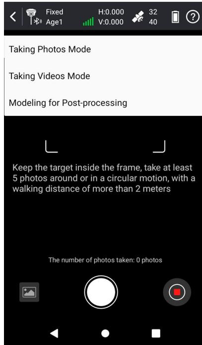
SOUTH's 3D modeling technology are fully utilized and transformed in INNO8. The results of image measurements by INNO8, can be seamlessly integrated with data outcomes from UAV. UAV surveys often face challenges of data gaps, leading to incomplete model outcomes. In such cases, surveyors can use INNO8 to collect image data on the ground and incorporate it into aerial survey data as a supplement, thereby enhancing the overall model outcome.
