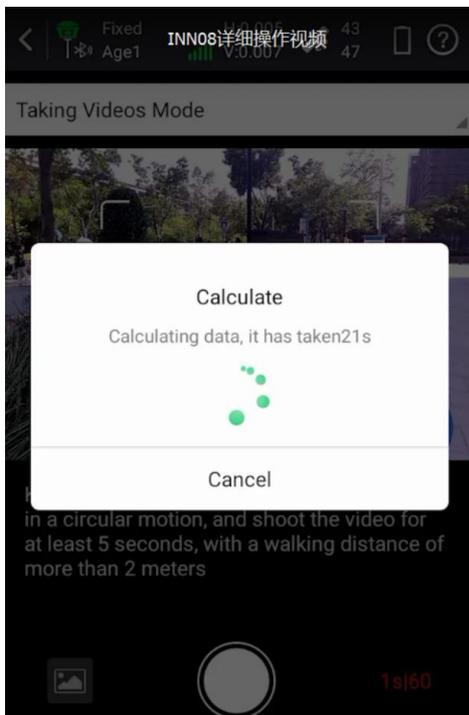
5) After the solution is completed, click OK, select three pictures, select the same target point, you can calculate the coordinates
