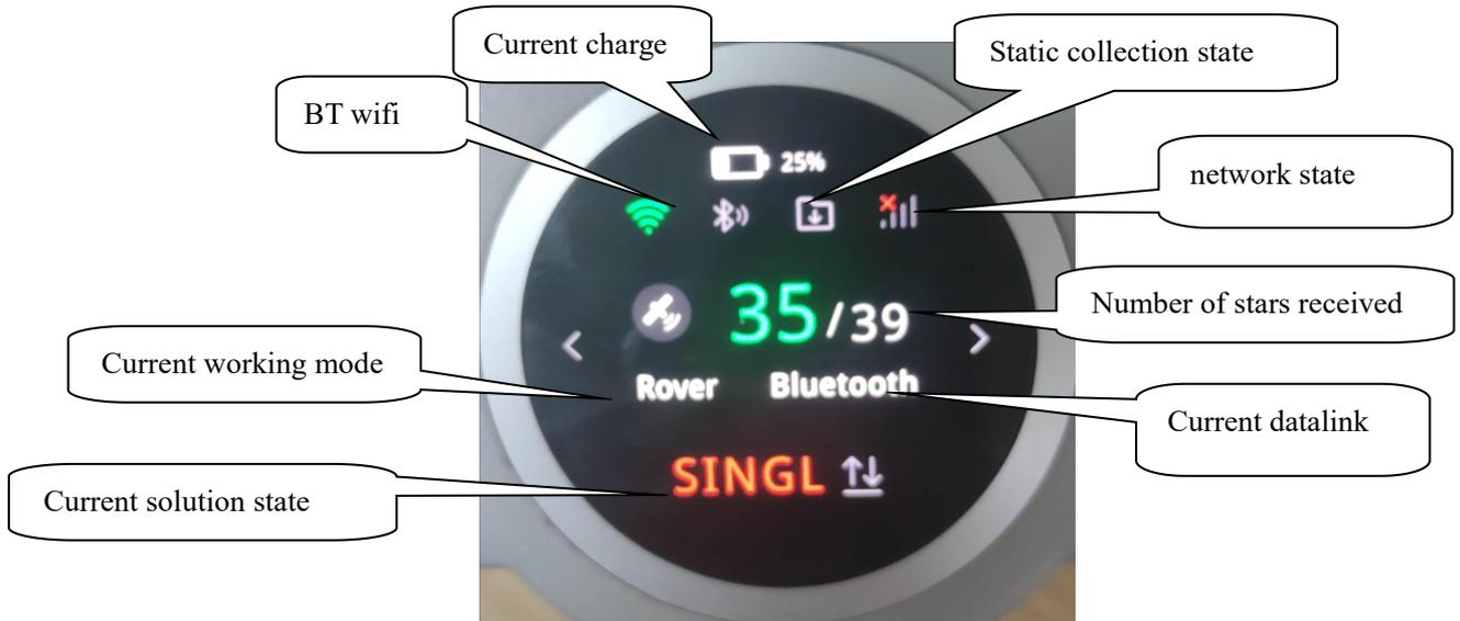
The LCD display is divided into main interface, first-level menu and second-level menu.
