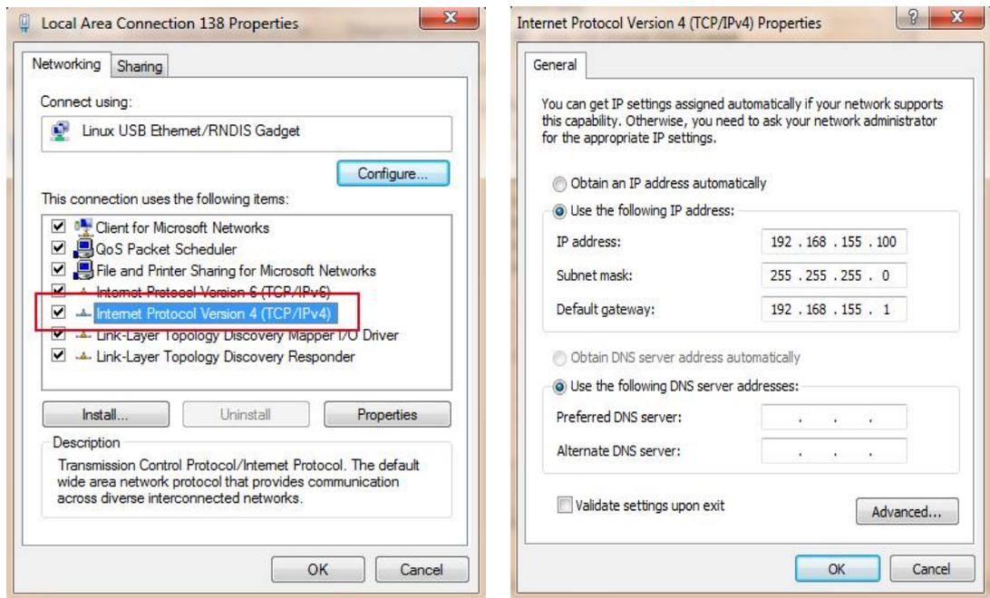
Run IE browser on computer and input the **default IP (192.168.155.155)** into address bar, after a while, the system login interface is refreshed, then apply **“admin”** for username and password to login.
