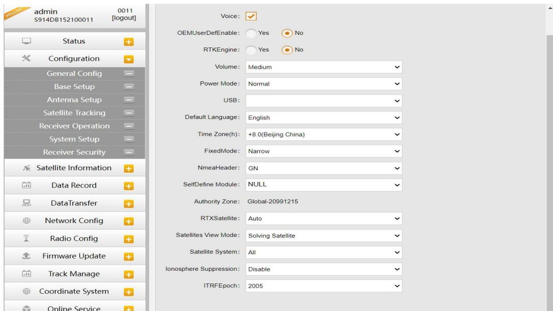
**Voice:** Check on this box to turn on the voice guide for INNO8, uncheck it to turn off the voice guide.
