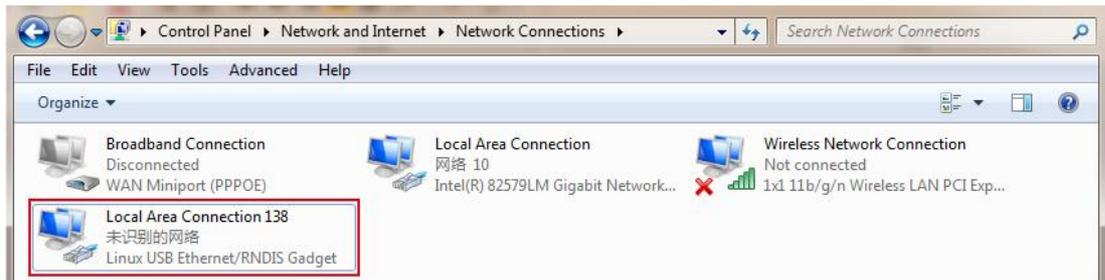
However, sometimes the computer cannot detect the receiver by USB network interface because there is something wrong with acquiring IP automatically, therefore, we need to do something to avoid such problem, that is to set a fixed LAN IP for the connection:
