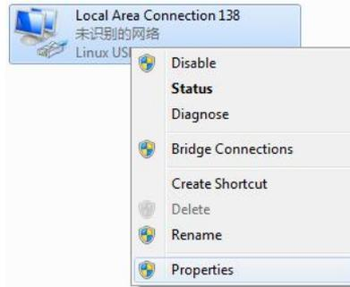
Then double click on Internet Protocol Version 4 (TCP/IPv4) option or click on properties button to call out Internet Protocol Version 4 (TCP/IPv4) properties window, set the fixed LAN IP address as shown in following, then click OK button and confirm the settings, return to the IE browser and use the IP address 192.168.155.155 to access the internal web UI.
